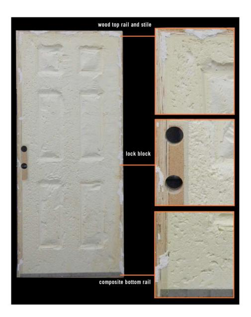
This model illustrates a fiberglass door with composite stiles and composite bottom rail. The top rail, however, is made of wood which leaves room for water to cause damage. The uneven surface results in density inconsistency and cause the skin to easily be peeled off.
