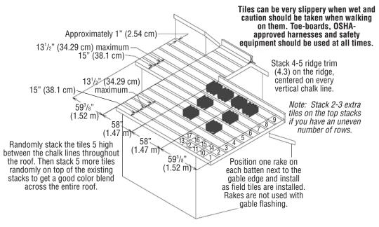
(1.47 m) O.C. on either side of that center line. Add extra stacks along the hip and valley to allow for one (1) tile per row to be cut on each side. Adjust the starting line to allow for proper rake fit at the gable.
