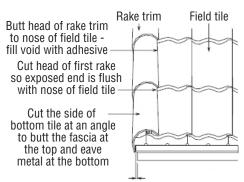
Eave closure and metal extends past end of fascia board and is cut at an angle to support bottom rake at same angle as the rest Grout is used to fill any openings
